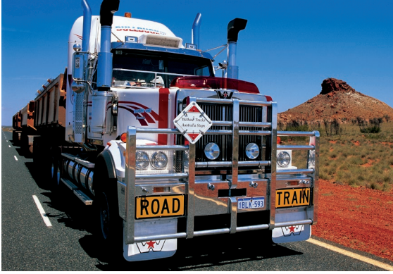
Australia Road Train with Cummins ISM carrying 120,000 lb load
