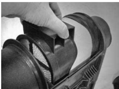
The PSD09, PSD10, and PSD12 filter can be easily removed with the built-in grab handle.
