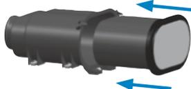
**6 Insert the primary filter.** For PSD08, slide the filter into the housing until the gasket seats against the housing. For PSD09, PSD10 and PSD12, slide the filter down at approximately a 5° angle until it hits the end of the housing. Rotate the filter toward the outlet section to complete the seal.
