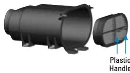
**3 Remove safety filter.** Using the plastic handle on the face of the safety filter, pull the filter toward the center of the housing and remove.
