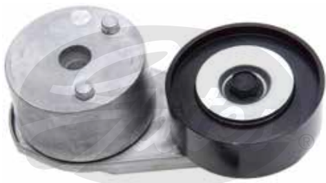
Pulley: O.D.: 86.5mm, Width: 32mm
