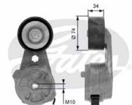
Pulley: O.D.: 74mm, Width: 34mm
