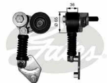
Pulley: O.D.: 65mm, Width: 36mm
