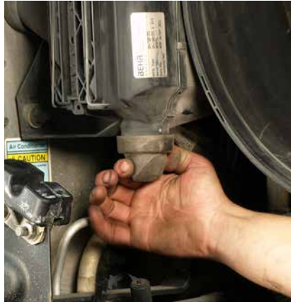
The Donaldson Vacuator™ Valve can be found on the majority of Donaldson air cleaners.
