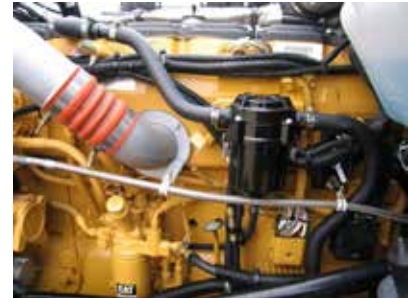
CCV4500 installed on a CAT engine.
