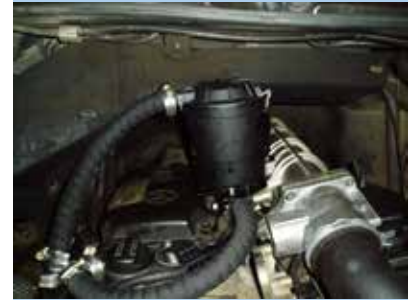
CCV4500 installed on a CAT engine.
