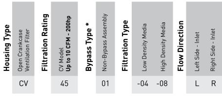
\* If plugged: Non-Bypass assemblies will experience increased pressure on oil pan and non-pressurized engine ports.
