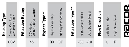
\* If plugged: Bypass assemblies allow aerosols to bypass the filter and reach the turbo.
