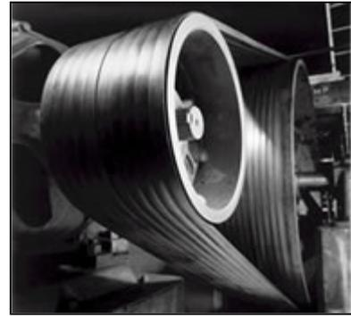
**Hogger Drive for Timber Industry** A hogger drive running five 5V 850 belts was burning through them every few months. When the belts failed, there was 1-2 hours of downtime to replace and re-tension the drive. After running KEVLAR® reinforced 5VP cross section Predator Singles belts on this application for 20 weeks, there was no noticeable wear.
