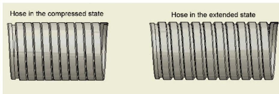
**Figure 1. Fully Compressed and Fully Extended Flex Tubing**
