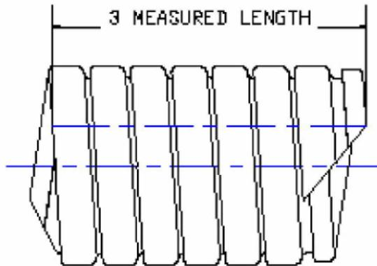
Figure 2. Measured Length and Open End to Right
